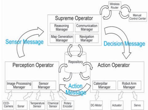
Fig. 2: Operational architecture of the robot
