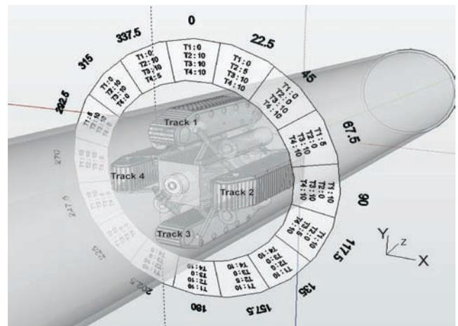
Fig. 3: Control architecture of the robot
