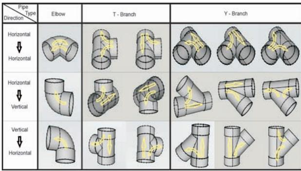
Fig. 4: Different types of motion in elbow, T-, and Y-branches
